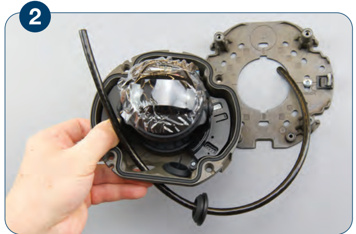
2 Insert cable stub through opening in camera.
